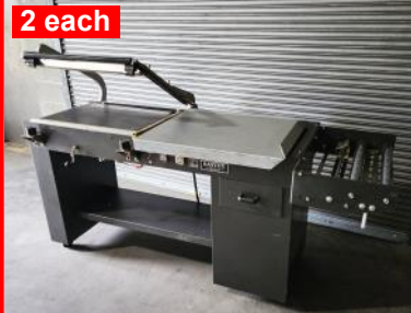
Eastey L-Sealer Model EM28T 28" x 20" Sealing Area
